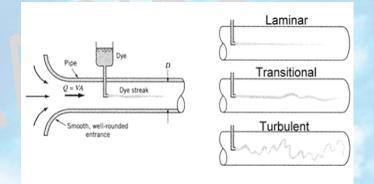
Laminar Flow (Re < 2300, only in pipe): Laminar flow may be described as an orderly pattern, i.e. in laminar flow the fluid moves in layer, or laminas, one layer sliding over an adjacent layer with only a molecular interchange of momentum. Such that the transverse exchange of momentum is insignificant.
