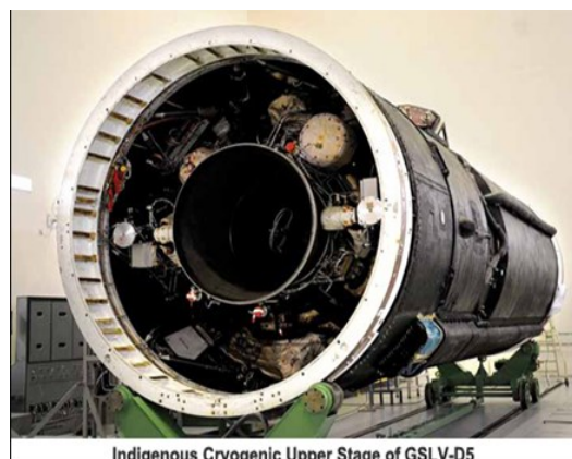
Indigenous Cryogenic Upper Stage of GSLV-D5
