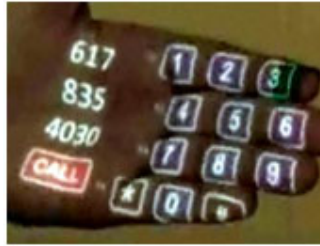
Fig. 5: Image Showing Dialer Projected on Palm to Make Calls Using Sixth Sense Technology
