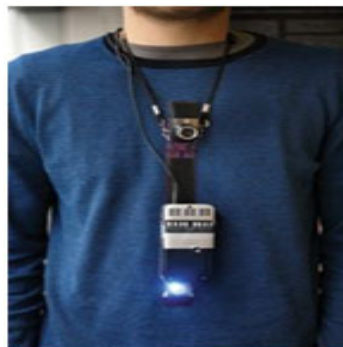
Fig. 2: Image Showing Sixth Sense Technology Prototype Equipped With Pocket Projector, Mobile Components, Mirror, Color Markers, and Camera
